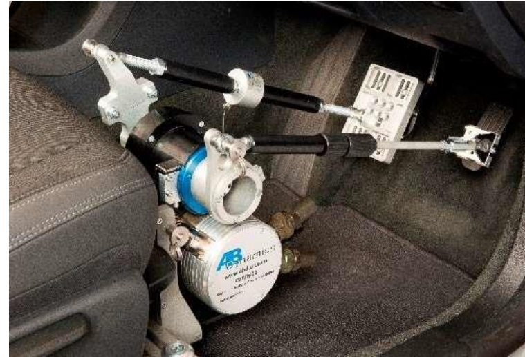
CBAR600 – COMBINED BRAKE AND ACCELERATOR ROBOT
